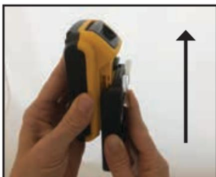
To remove the battery cartridge from the holster, press the release button and firmly pull the battery cartridge out of the holster.
